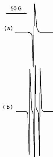
Fig. 5. ESR spectra of: (a) chloranil semiquinone free radical ( g = 2.0038 ), and (b) after adding 2-methyl-2-nitrosopropane ( g = 2.0050 , \mathcal{A} 16 G).
